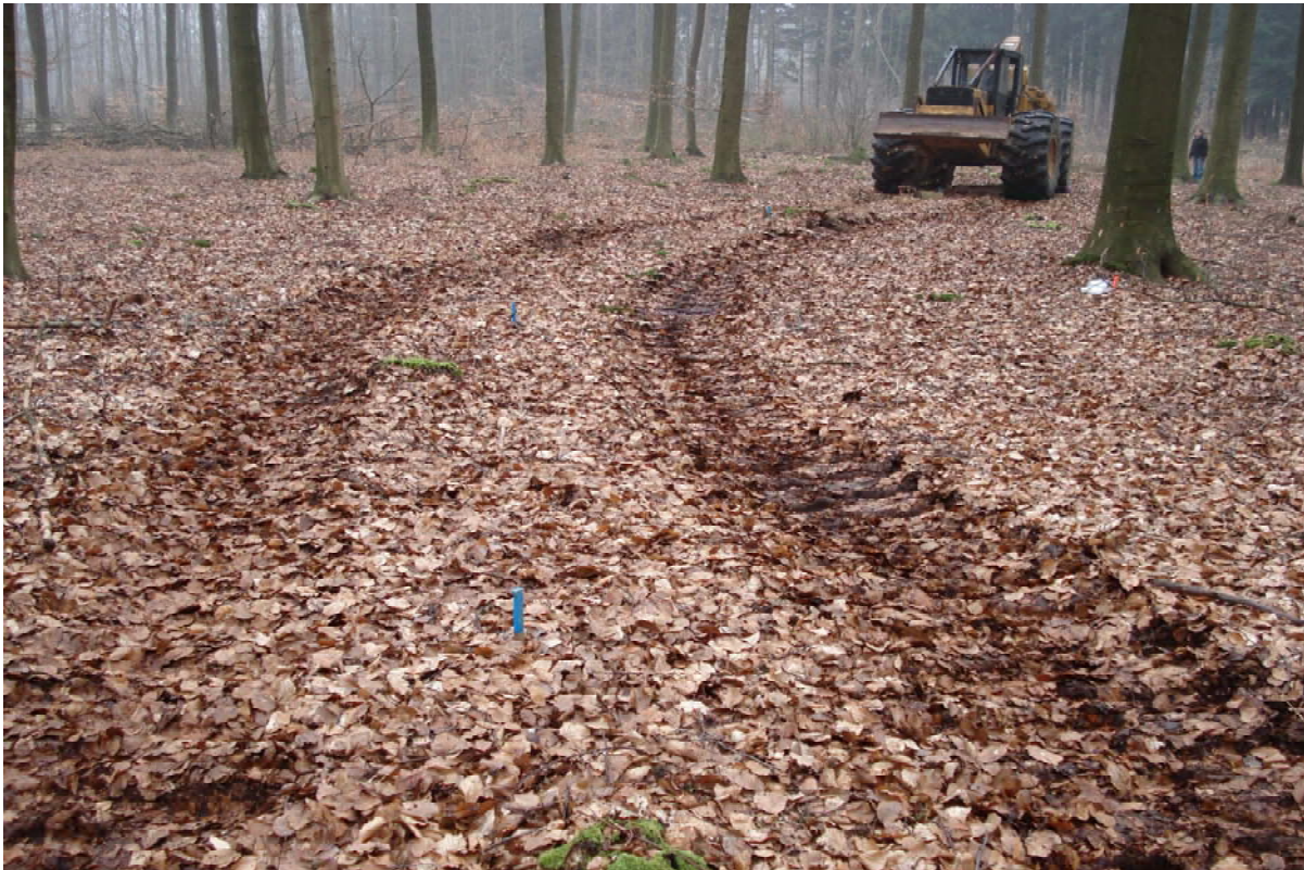
Painted sticks indicated the centres of the experimental skid trails at the field trial in Meerdaal forest (Leuven) (Chapter 2), in order that the machines would follow the same tracks at subsequent passes. The photograph shows the skid trail where a John Deere grapple skidder JD 640 made five passes back and forth in February [photograph: Lotte Van Nevel, February 2007].
