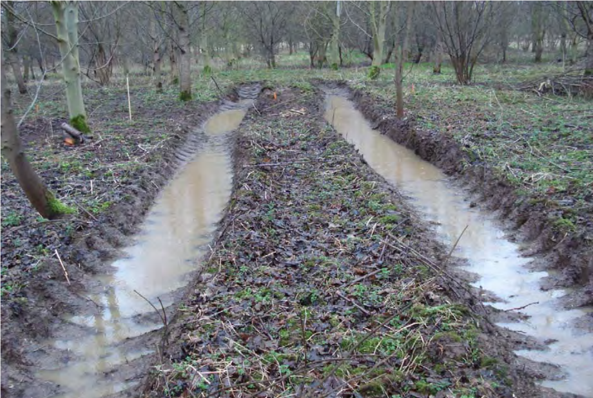
Water stagnation in deep ruts caused by five passes of the John Deere grapple-skidder JD640 at the field trial in Walem 1 (Chapter 2) [photograph: Evy Ampoorter, February 2007].
