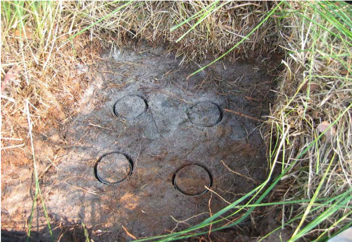
Four Kopecky cores, brought into the soil for determination of the bulk density of depth interval 0-10cm (Chapter 3) [photograph: Robbie Goris, August 2004].
