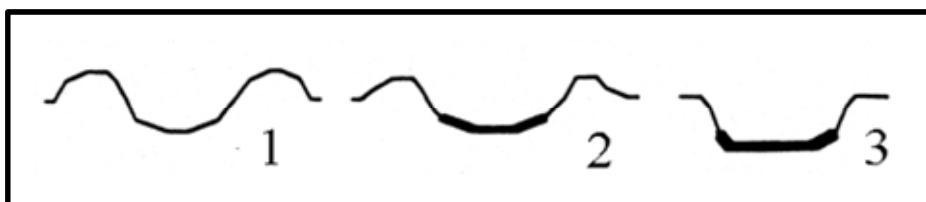
Fig. 1.3 Rut types (Abeels 1989): rut type 1 is caused by plastic deformation, rut type 2 by a combination of plastic deformation and soil compaction and rut type 3 by soil compaction only.
