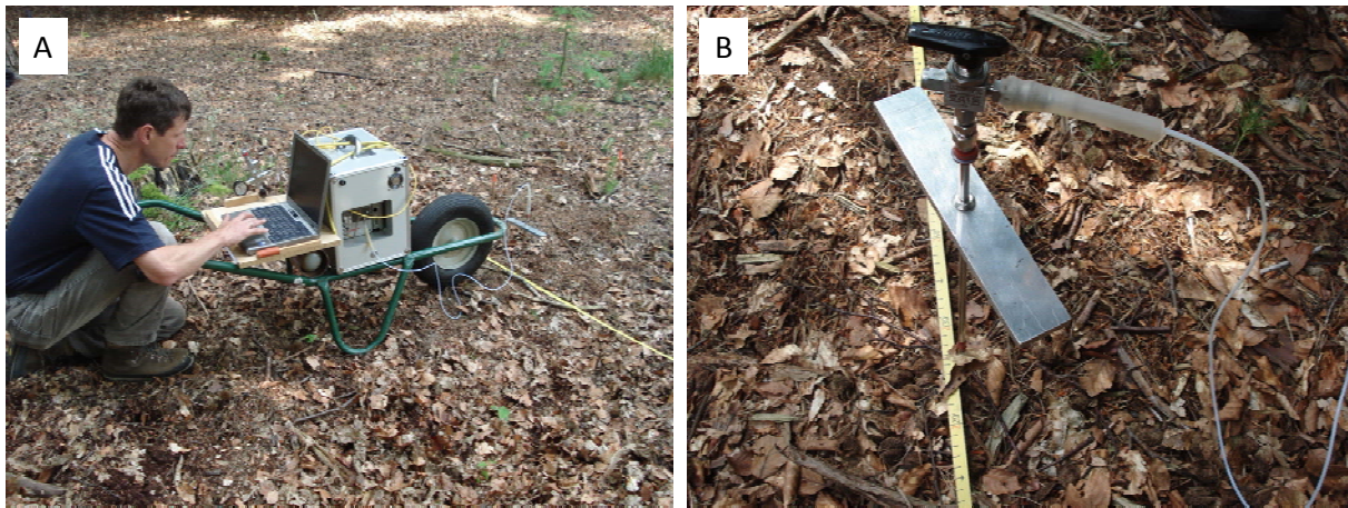
Fig. 2.4 Quantification of soil CO 2 concentration: (A) portable gas chromatograph, (B) detail of needle [photographs: Evy Ampoorter, June 2008].
