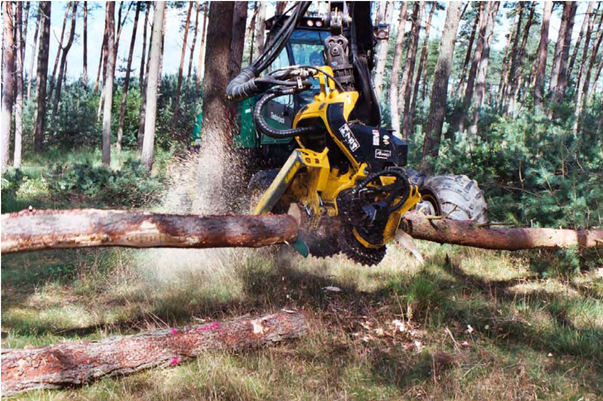
Detail of the processor head of the Timberjack 1070D harvester, used in Putte (Chapter 3) [photograph: Robbie Goris, August 2004].
