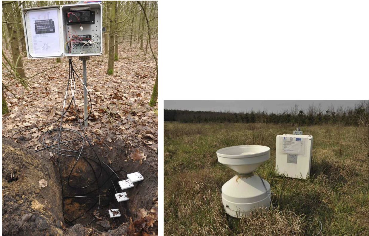
TDR probes at 5, 15, 30 and 50 cm depth (left) and the tipping bucket (right). Both connected to a datalogger
