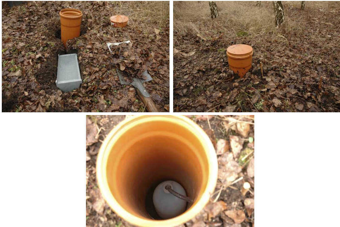
Installation of a zero-tension lysimeter (upper) and sampling of the forest floor leachate (lower)
