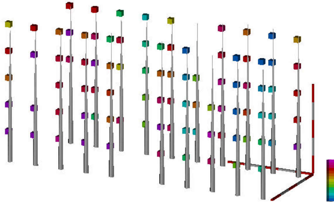
Fig. 46. Cd concentrations at the sampled locations within the studied stand. Cd scale ranges linearly from 1.1 (blue) to 14.3 mg.kg -1 DW (purple); the markers show the origin of the longitudinal axis and represent 5 m, a single unit 1 m. Stand is shown from a North-eastern view.
