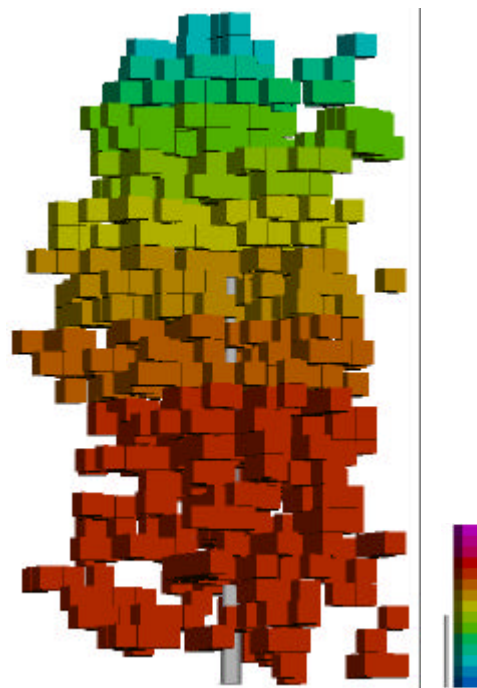
Fig. 18. Cd concentration calculated with deterministic trend given by equation [3.7] at all possible sampling unit locations. Scale ranges linearly from 2.4 (blue) to 10.7 (purple) mg.kg -1 DW; the grey bar next to the color scale represents a height of 1 m (North-western view) n = 1136
