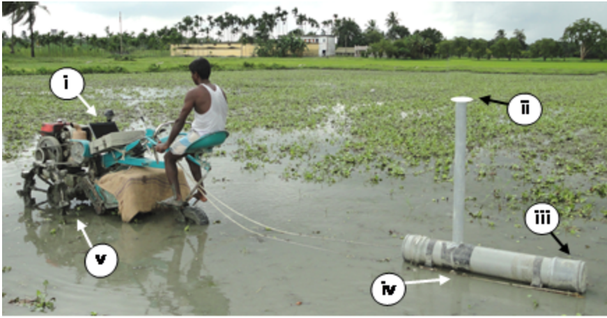
Fig. 2. The Floating Soil Sensing System (FloSSy) during field measurement of apparent electrical conductivity ( EC_a ). The different components are indicated as: (i) laptop, (ii) GPS, (iii) water proof sensor housing, (iv) floating platform, and (v) the power tiller.
