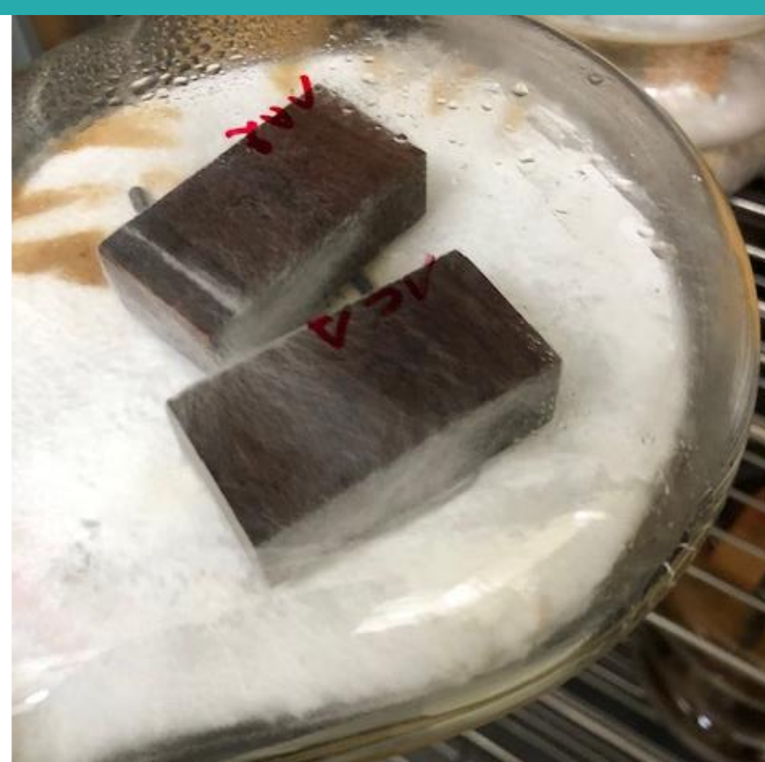
Two thermally treated wood samples during a fungal degradation test
