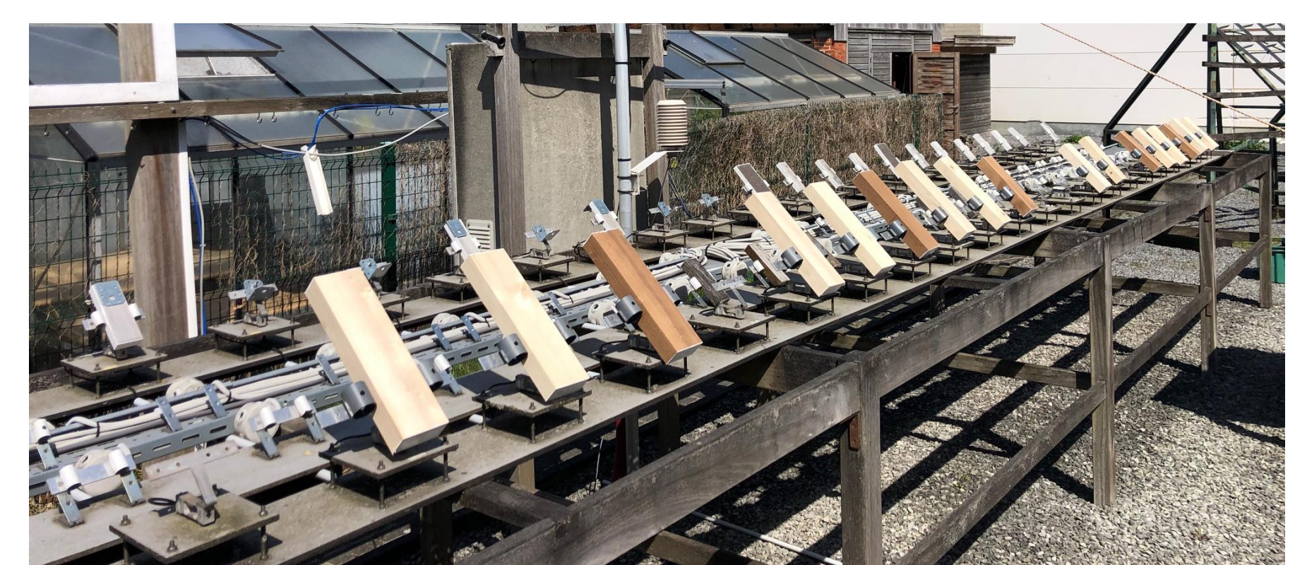
Figure 4. Continuous moisture measurement (CMM) set-up
