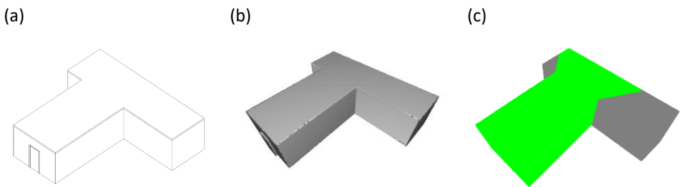
Figure 4.6. The 3D visualization of the (a) geometrical model from as-planned BIM, (b) detectable model, (c) classified detectable model.
