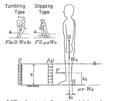
Figure 5 Effect of overtopping flow on the static balance of a person
