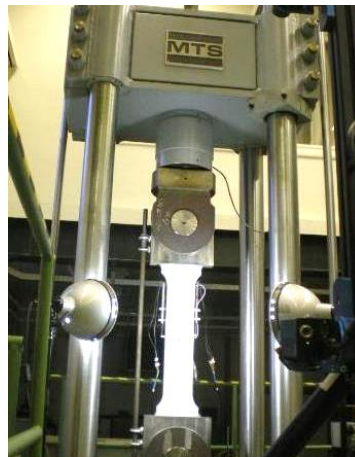
Figure 2: Medium Wide Plate tension test
