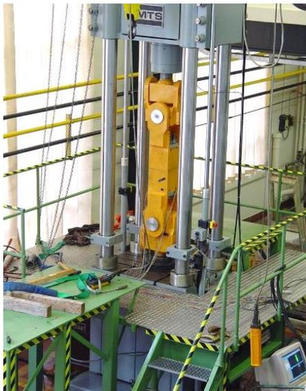
Figure 1: MTS load frame
