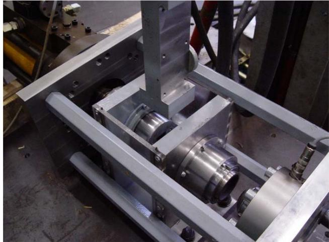
Both friction material specimens are placed in holders, which fit into the wall of the test-box, mounted on the bottom plate of the load-frame. The specimen holders can slide in the horizontal direction to accommodate wear of the friction material specimens. The test box itself is sealed such that it can be filled with a lubricant or with (sea) water to simulate as close as possible the working conditions of the application.
