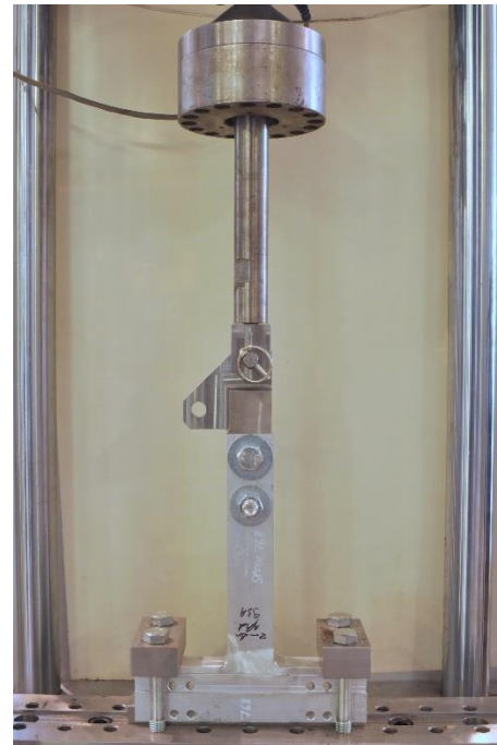
Figure 2: Fatigue testing of welded aluminum T-joint
