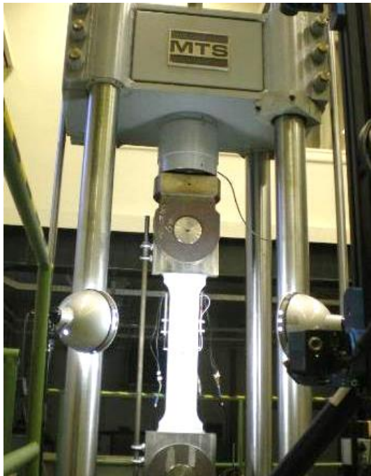
Figure 1: Medium wide plate tension test in MTS 2500
