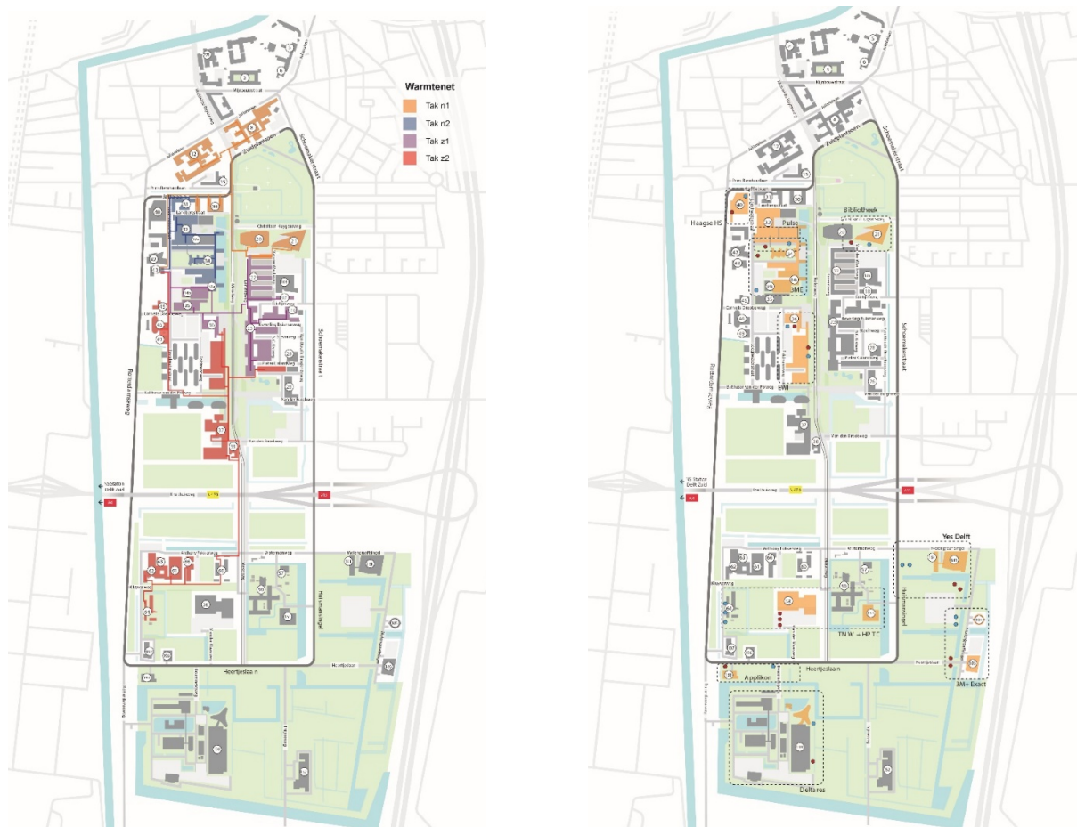
Figure 12.03: Map of TU Delft with buildings connected to HT heat network (left) and current ATES systems (right)
