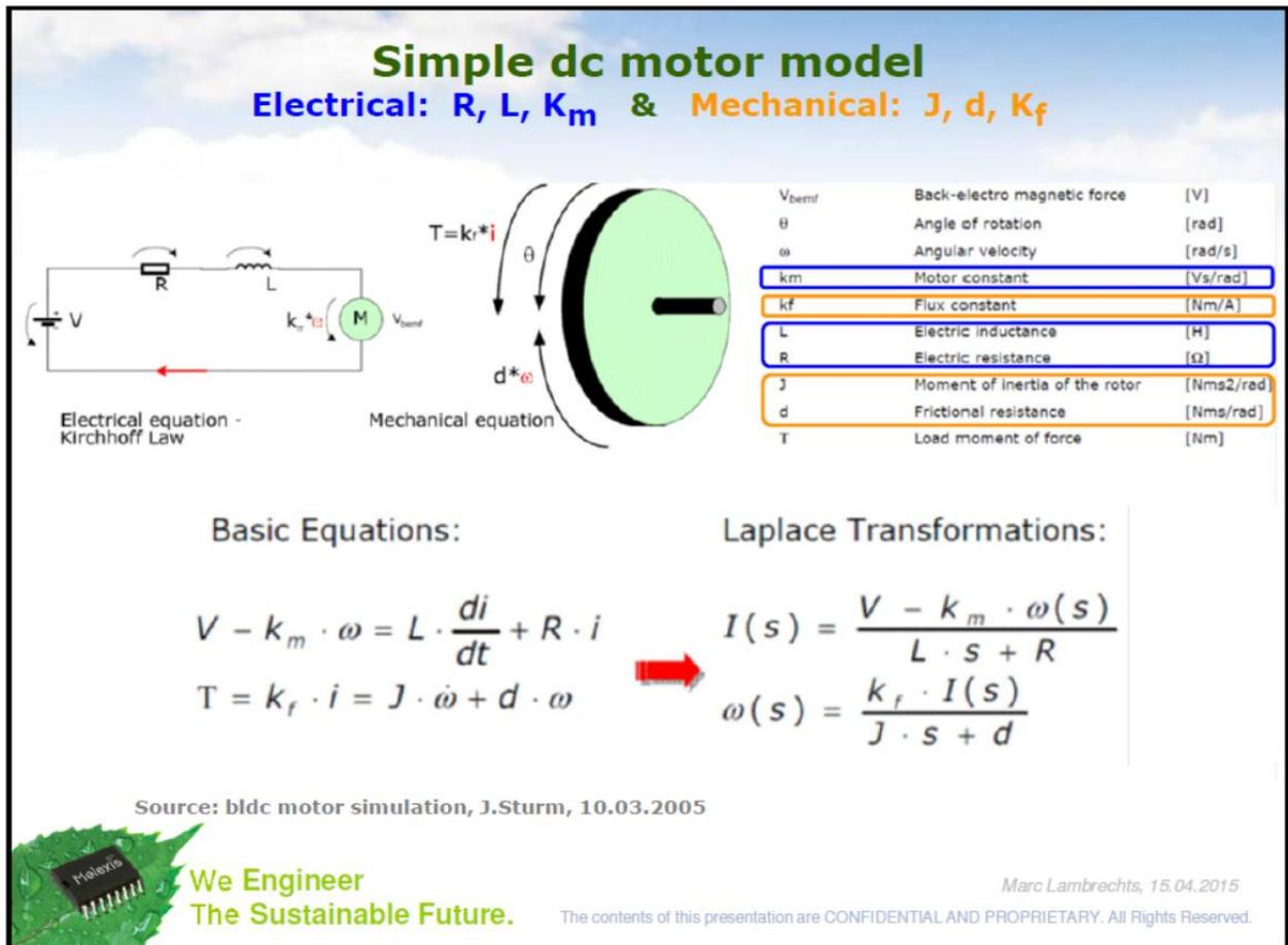
Fig 1: electro-mechanical model for a motor system
