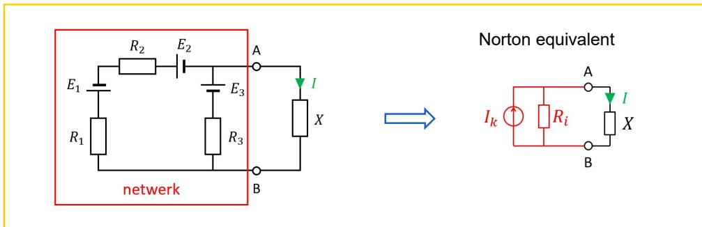
$$I = \frac{R_i}{R_i + X} I_k \quad \Rightarrow \quad I_1 =$$
