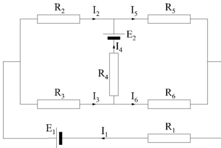
$$\begin{aligned} R_1 &= 1 \Omega \\ R_2 &= 20 \Omega \\ R_3 &= 30 \Omega \\ R_4 &= 0,5 \Omega \\ R_5 &= 30 \Omega \\ R_6 &= 20 \Omega \end{aligned}$$
