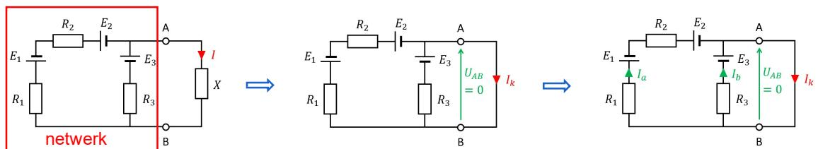
$$U_{AB} = E_3 - R_3 I_b = 0 \Rightarrow I_b =$$
