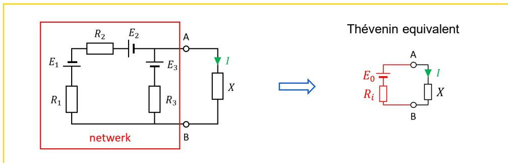
$$E_0 = (X + R_i) \cdot I \quad \Rightarrow \quad I = \frac{E_0}{X + R_i} \quad \Rightarrow \quad I_1 =$$
