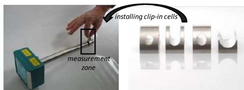
Figure 3.6. Picture of the Parsum probe (left) and the clip-in cells (right, top-view).
