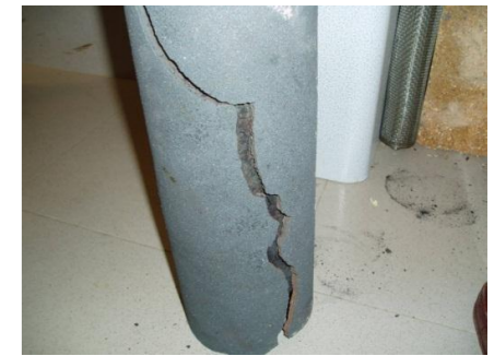
Hot spots due to inhomogeneous coke formation
