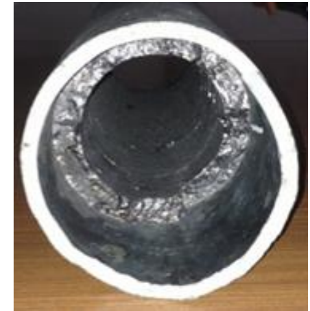
Coil cracking due to differences in thermal expansion rate
