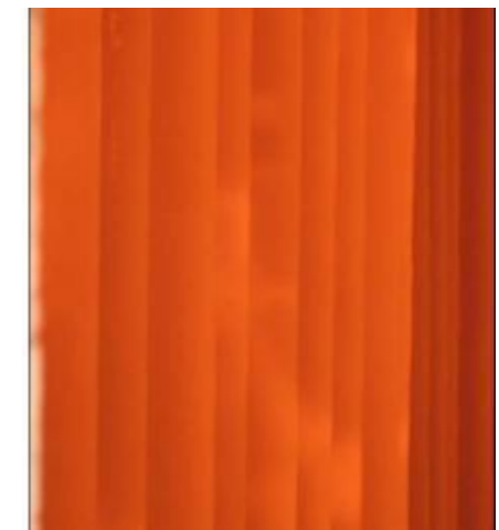
Hot spots due to inhomogeneous coke formation
