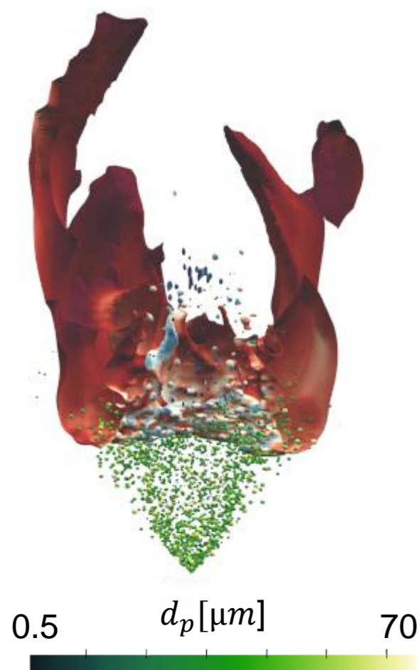
Stoichiometric mixture fraction iso-contour colored with the instantaneous Temperature
