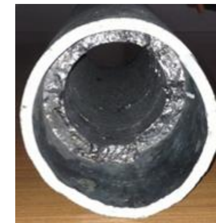
Coil cracking due to differences in thermal expansion rate
