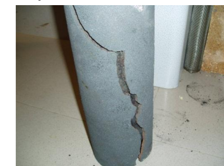
Coil cracking due to differences in thermal expansion rate
