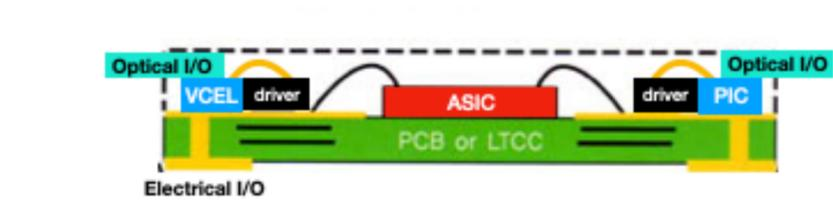
**Multi-Chip-Module (MCM) or System in Package (SiP)**
