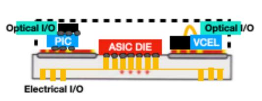
**2D System in Package (SiP) & hybrid Photonics**
