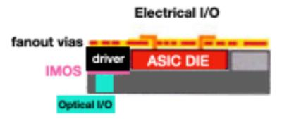
**2.5D multiple die Wafer Level fan-out package & photonics with integrated electronics (IMOS)**
