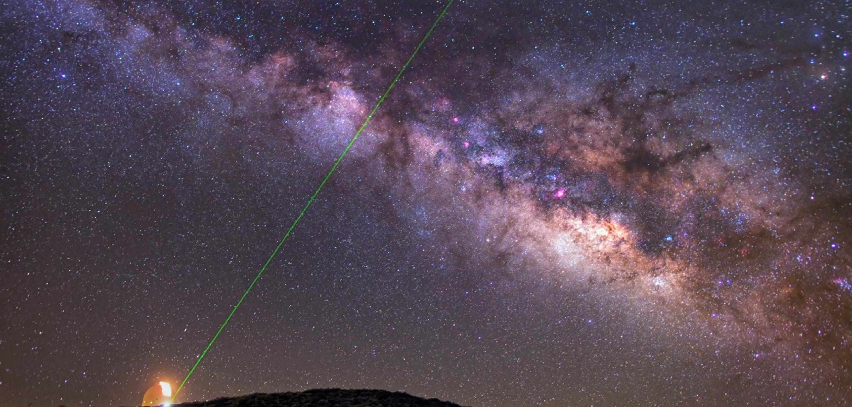
Laser Guide Star needed for PAA atmospheric measurement (i.e. creates a fake star were the satellite is going to be to measure the distortion for the uplink)
