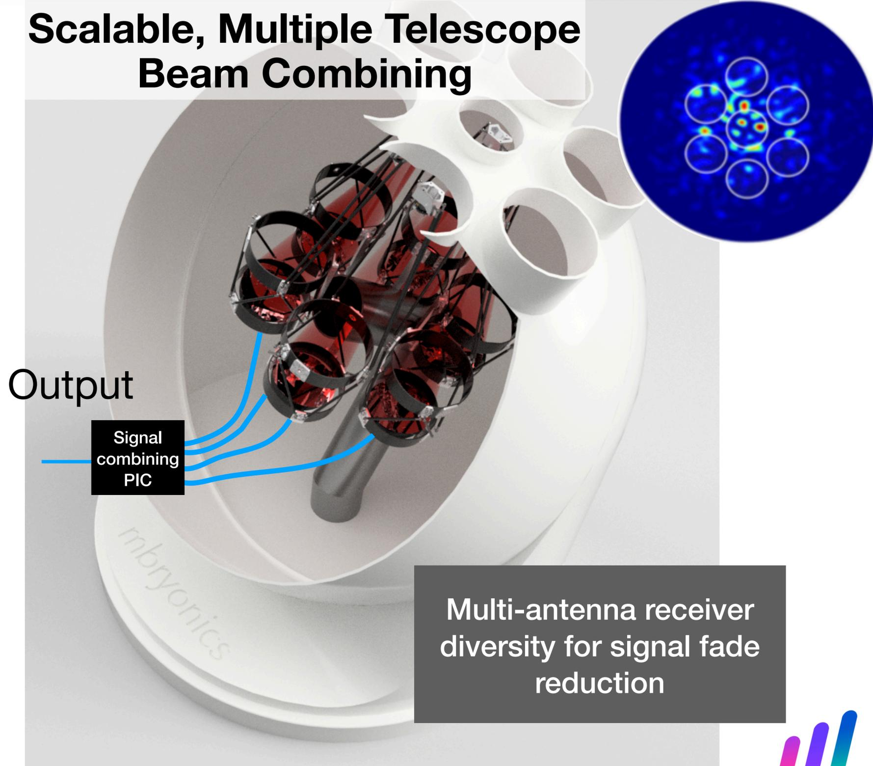
Multi-antenna receiver diversity for signal fade reduction
