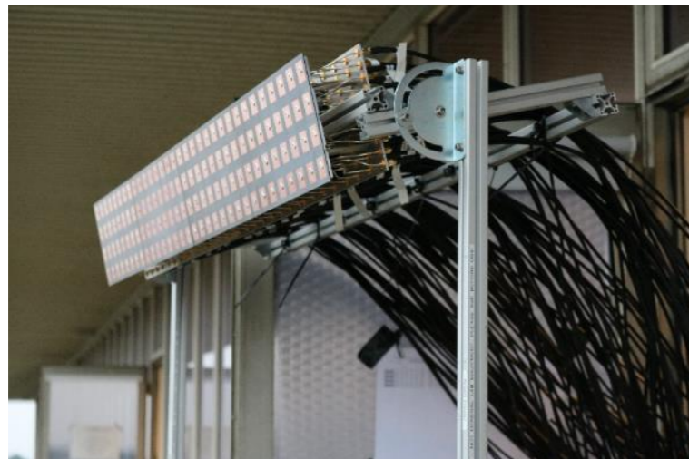
Massive MIMO array with electrical routing
