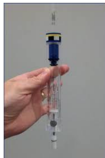
Figure 2. Sample, spinner, and depth gauge used to prepare an NMR sample
